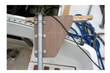
The top of the leg is supported by a crosspiece and a plywood support.
