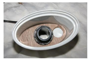
After some gentle sanding and adjustment, I assembled it using Sikaflex as a sealant between the plastic and the wood.
