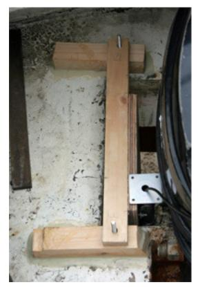
The whole assembly is held tight by 2 M8 wing nuts which are bolted into the bearers.
